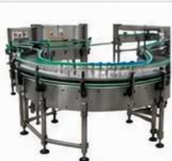
Bottle Conveyor System
